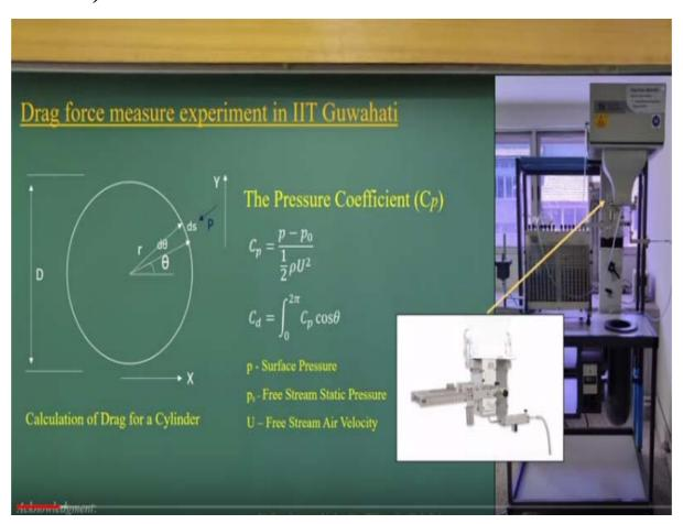
I am to just show you that there was an instrument which can measure the drag force measurement experiment set up like these where you can compute the pressure co efficient and if you integrate it in get the drag co efficient and that way when you have put a cylinders you can compute the what could be the drag the force acting on these cylinders with the varying the fluid flow the air flow conditions here.
