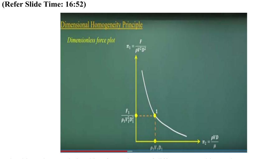
I should conduct a relationship of experiment of different Reynolds numbers and can get it from the experiment but we need the force and non dimensionless as a  $F_1$  functions and void heat wave functions getting these. So only 10 experiment are enough for this study as compared to conducting the 1000 experiment. So the non dimensionless experiments making us that we can make a dimensionless force plot.
